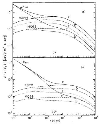
Fig. 5. – Differential energy muon spectra for vertical (a)) and horizontal (b)) directions. Muons from  $\pi$ - and K-decays are considered according to the work  $(^{\circ})$ . Prompt muons are calculated in RQPM and MQGS for two variants of primary spectra. Pointed curves: spectra calculated in RQPM under the assumption of Feynman scaling (with the using of  $f_{c}^{\text{s(mod)}}(x)$ ).
