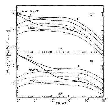
Fig. 6. – Total differential spectra of muon neutrinos and antineutrinos for vertical (a)) and horizontal (b) directions. Neutrinos from  $\pi$ - and K-decays are considered according to the work  $(^{\circ})$ . Prompt neutrinos are calculated in RQPM and MQGS for two variants of primary spectrum. Dotted curves: spectra calculated in RQPM under the assumption of Feynman scaling.
